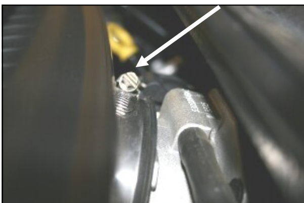
7. Using the 5/16" socket, ratchet and extension (or flat blade screw driver)- loosen hose clamp on the throttle body. This clamp is located close to the fire-wall, in the center of the engine compartment.
