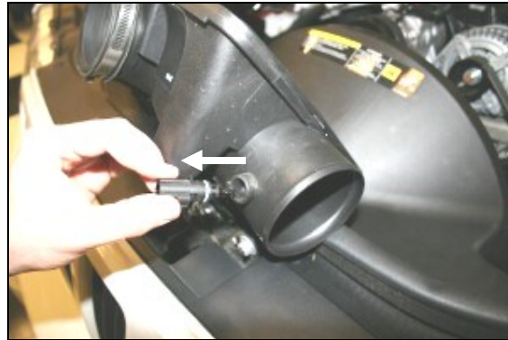
14. Remove the factory intake air temp sensor from the resonator box by carefully twisting the sensor body, and pulling it straight out of its mount. Place the sensor in a safe location, it will be re-used in step #15.
