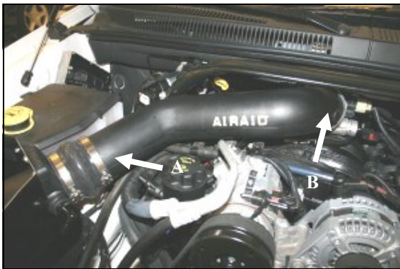
16. A.) Install the Modular Intake tube into the hump hose end first. B.) Insert the opposite end of the Modular Intake tube into the reducer, on the throttle body. Adjust components for fit, and then tighten all of the hose clamps, and reconnect the factory intake air temp sensor wiring harness.
