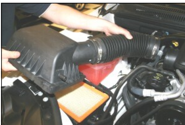
4. Remove the air cleaner lid, and factory intake tube from the resonator box.
