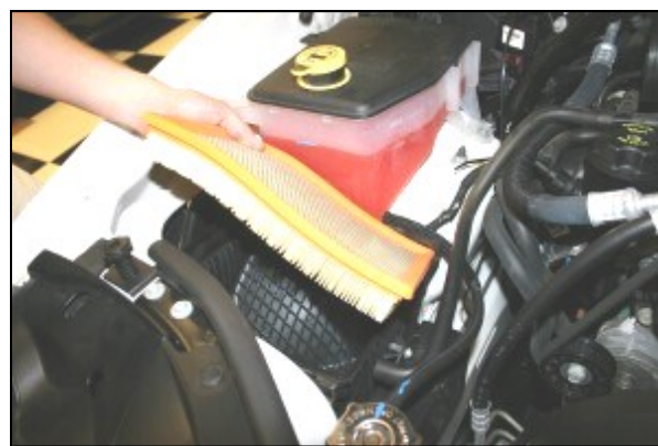
5. Remove the factory air filter.
